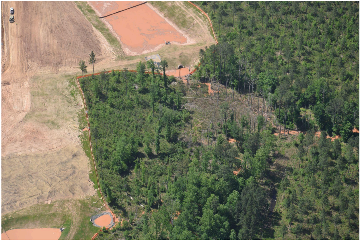
Attachment 8- Outfalls from dewatering operations at Vinfast in Chatham County, draining into wetlands feeding Shaddox Creek.
